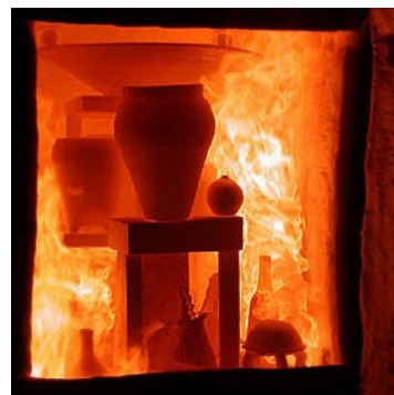
Clay being bisque fired to 1080°C in a kiln.
