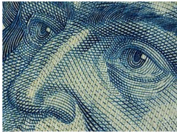
Intaglio is an engraving process used to print multiples of an image. A bank note is a good example of intaglio printing.
